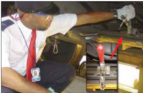
Figure 1-13 – Release folding stairs hold-down clamp
