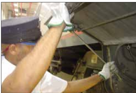
Figure 1-11 – Secure the door safety bar
