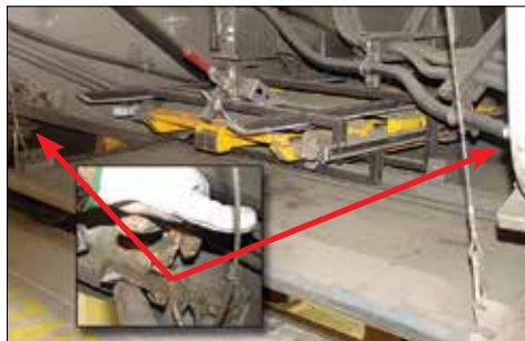
Figure 1-12 – Lower storage compartment latches and safety cables
