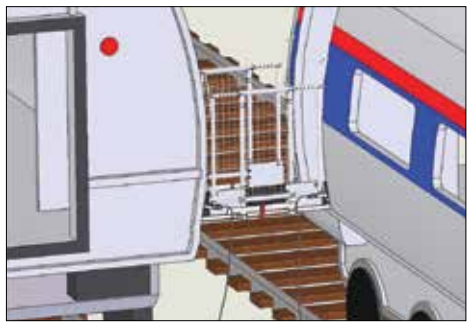
Figure 1-9 – Assemble railing and attach to railing post holder mounts as shown.
