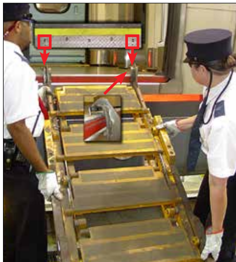
Figure 1-14 – Secure folding stairs to car body
